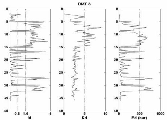
Figure 7. Typical DMT results at case 3 location. Estimated fill thickness at this point: 6 m.
