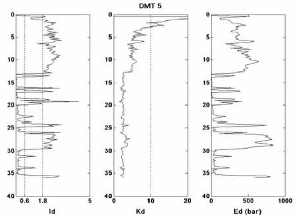
Figure 6. Typical DMT profile at Case 2 location
