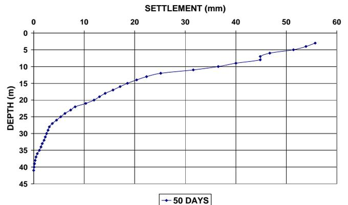
Figure 15. Last valid reading of the extensometer in Case 3.
